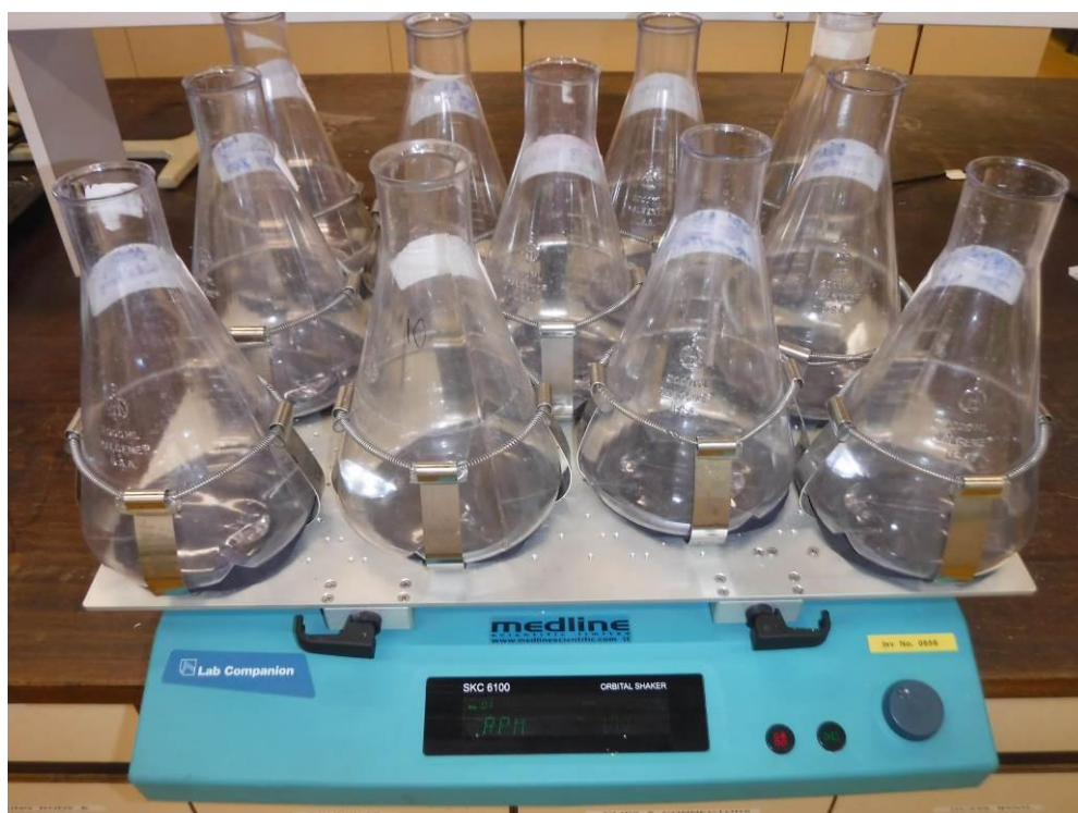
Photograph C 1 Orbital shake table
