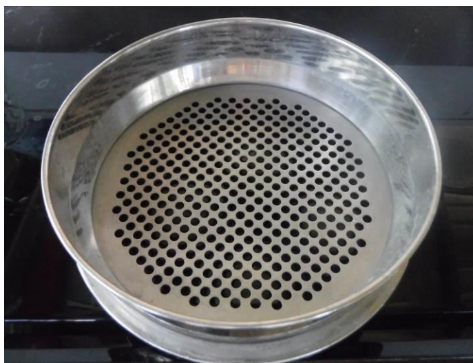
Photograph E 1 5.6mm perforated plate sieve
