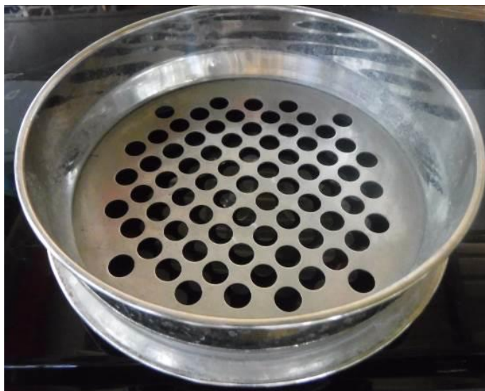
Photograph C 3 12.5mm perforated plate sieve
