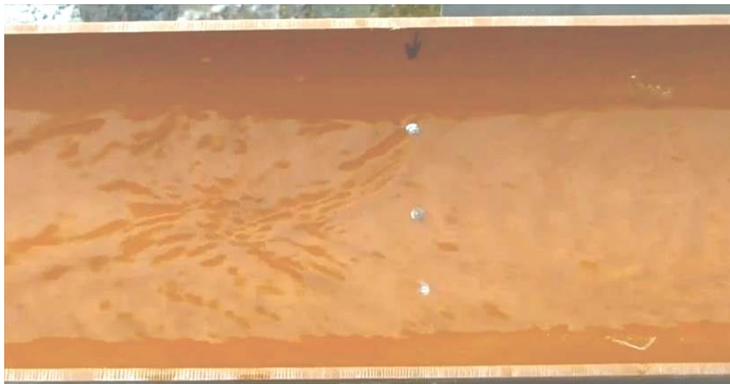
Photograph D 1 Snag points set in half radius 100 mm diameter pipe
