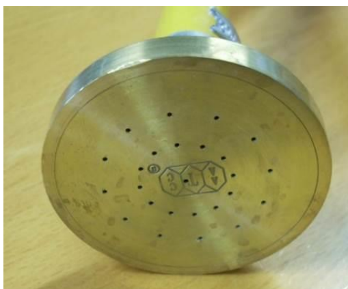
Photograph C 4 Standard test rinsing head
