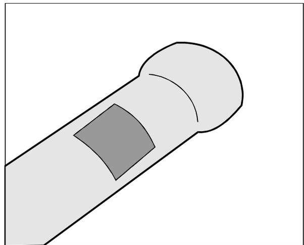
**Figure 22 - Clean and dry area to be repaired**
