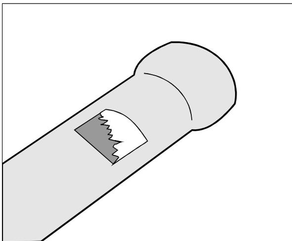
**Figure 20 - Sleeving damage to be repaired**
