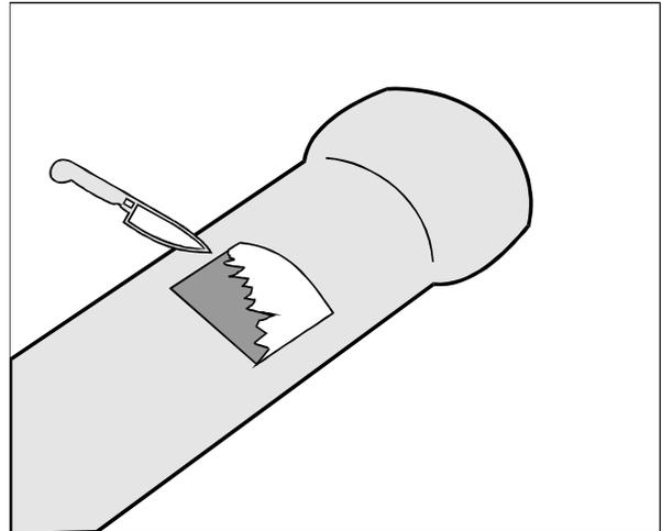
**Figure 21 - Cut away flap of material**
