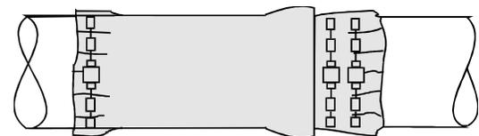
**Figure 19 - Completed joint protection****B2.3 Cutting pipes**
