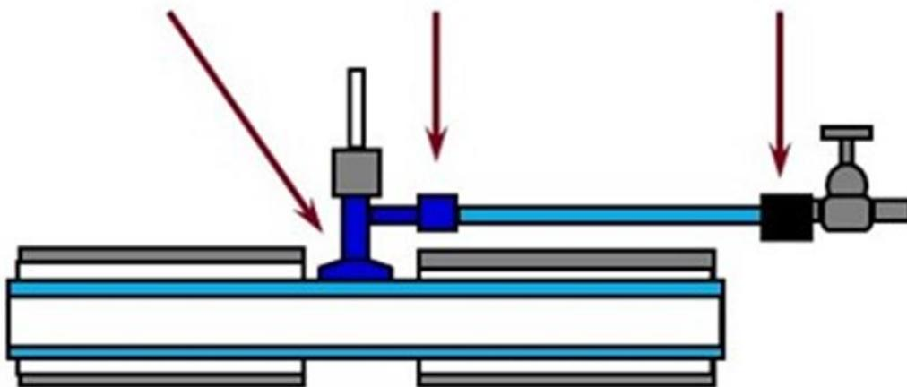
**Figure 6: Joints which could be assessed using the test for service connections**
