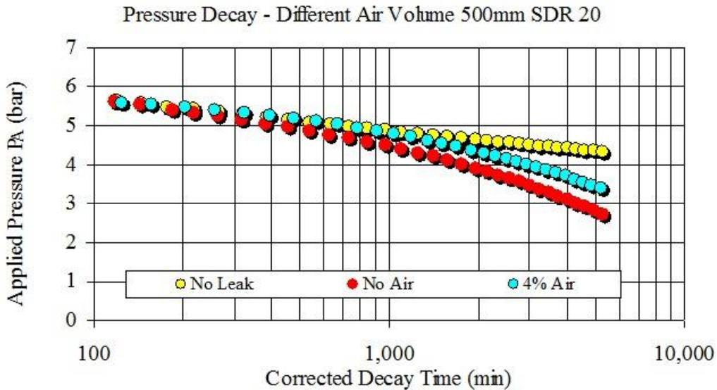
Figure B2: Effect of air on pressure decay in a PE Main with (a) No Leak and with (b) Leakage at 4 \* Allowable Rate
