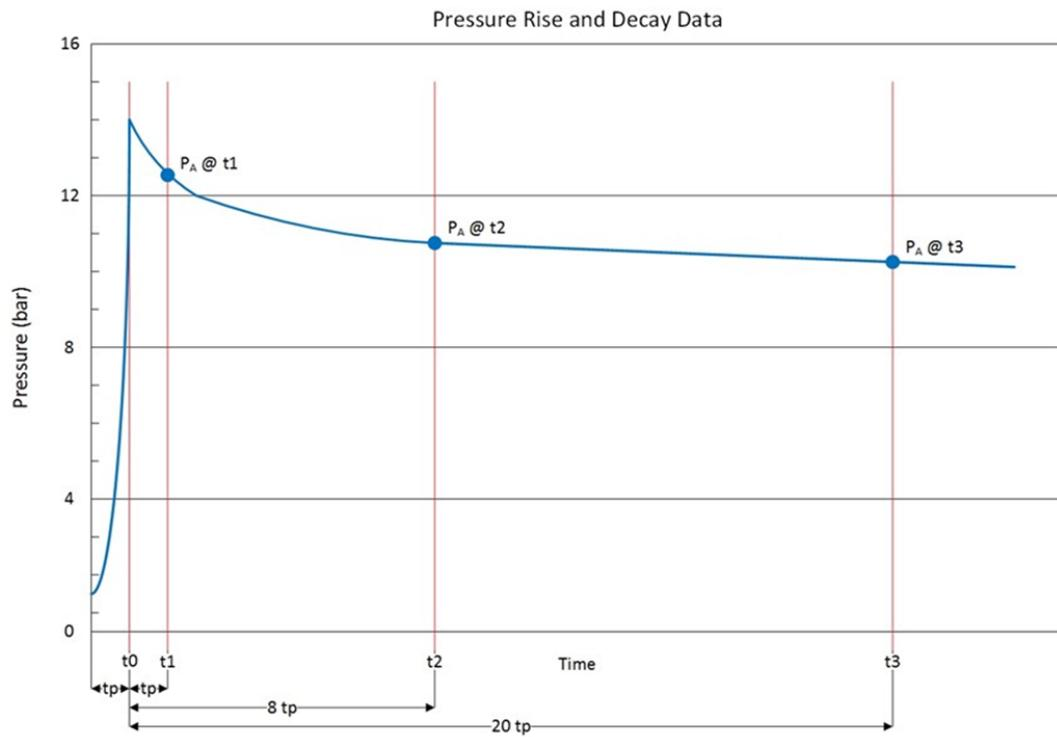
**Figure 3: Response of pressure v time for a PE pipe showing the times at which pressure values are analysed to determine the “n” values**
