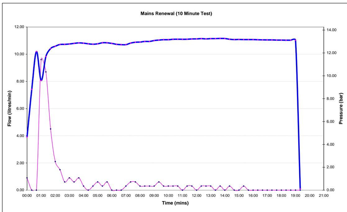
**Figure 4: Typical graph for acceptable renewed mains test showing pressure increasing with high flows, reducing as the test pressure is reached and decreasing as the rate of creep slows.**
