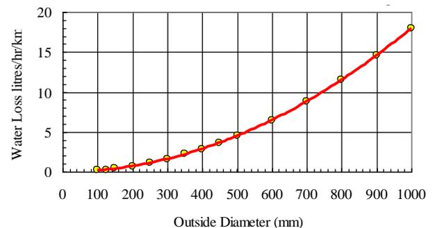
**Figure C1 Allowable Leak Rates for ductile iron with a Pressure Loss of 0.2 bar/hr.**
