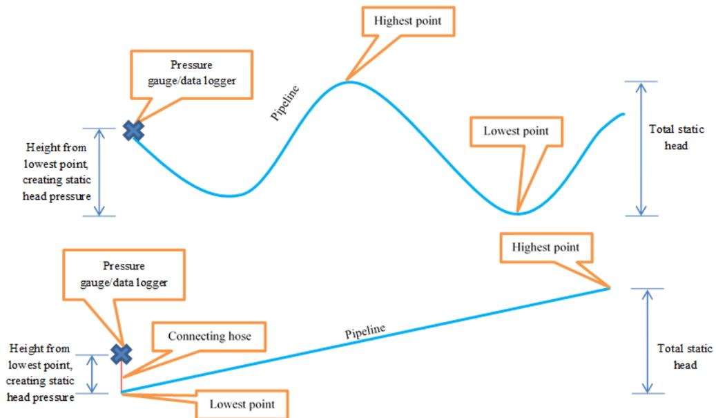
**Figure 2: Diagram showing correction for static head where test point is above the lowest point of main**
