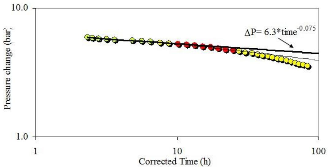
Figure D3: Raised Pressure ( $P_A$ ) v Corrected Time (on logarithmic axes) for a PE Pressure Test
