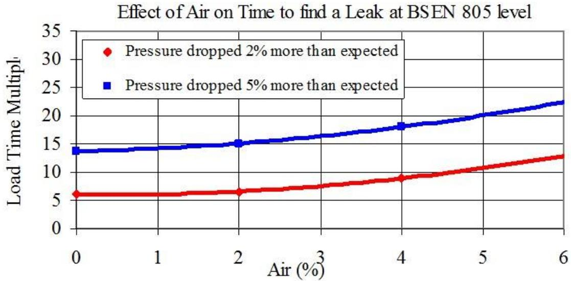
Figure B3: Effect of air on time (multiple of loading time) to detect a leak at BS EN 805 level
