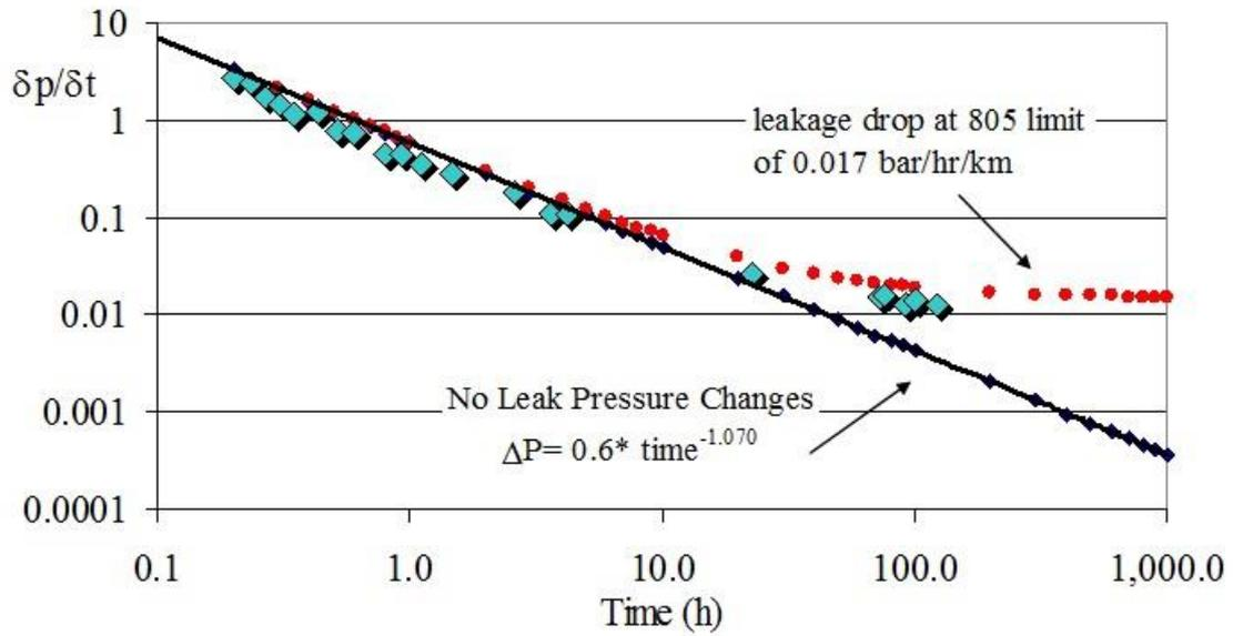
**D4: Rate of Pressure Decay as a function of Time for a PE Pipe (log axes)**
