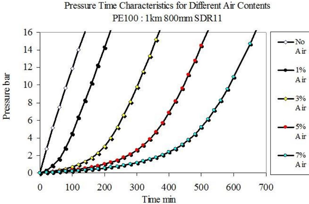
Figure B1: Pressure rise characteristics for 1 km of 800mm SDR 11 PE 100 Pipe
