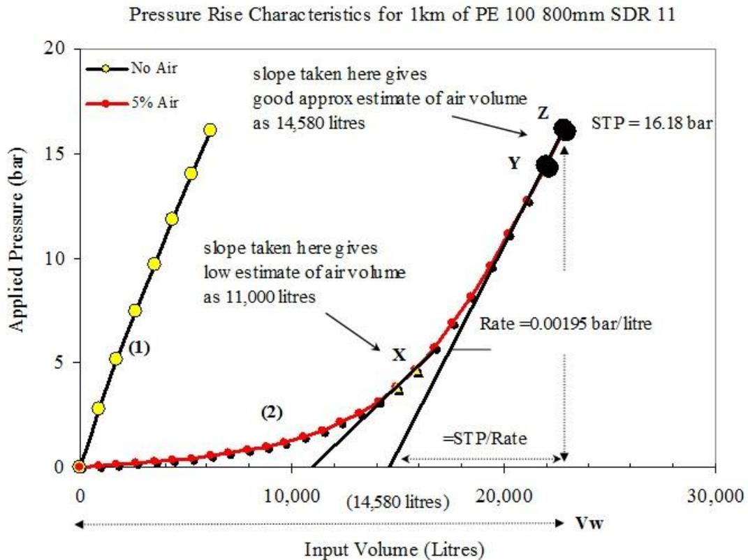
Figure B4: Pressure v Vol for (a) No Air and (b) 5% Air - 1km: 800mm SDR 11 Pipe
