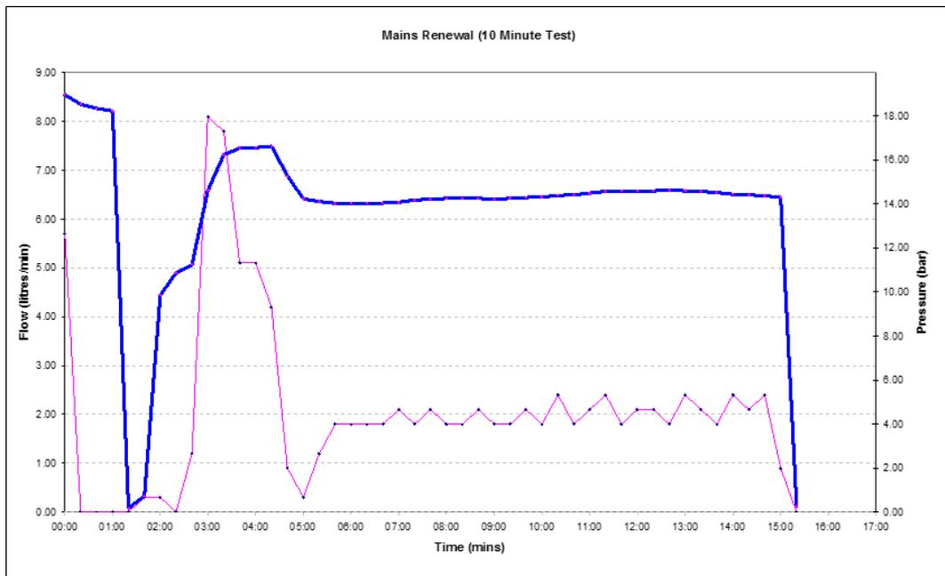
**Figure 5: Example graph for unacceptable renewed mains test indicating a leak - pressure fluctuates from the test pressure, flow rate is high and does not reduce over the duration of the test.**
