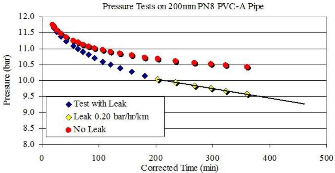
Figure D2: Pressure Decay Curves for PVC-A Pipe: with and without leaks
