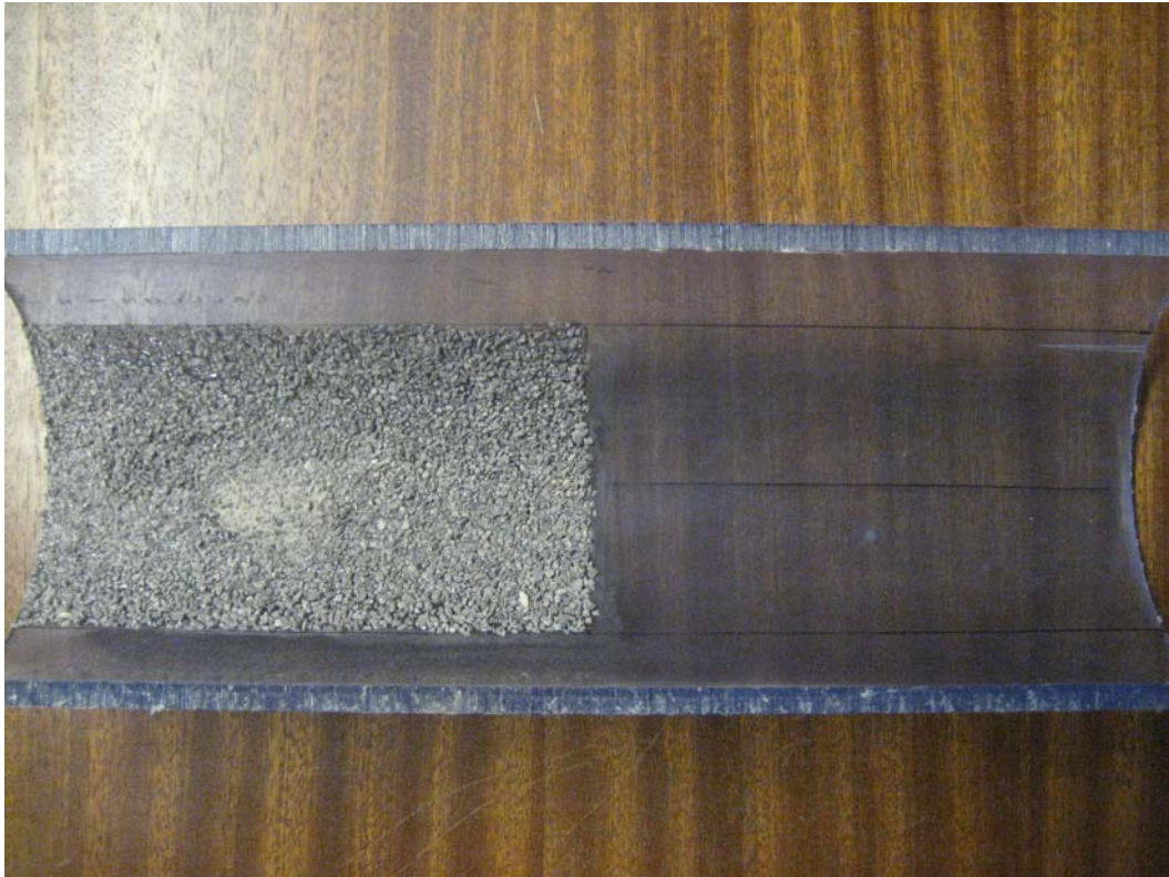
Figure 3.1 An example of 100 mm diameter pipe section with fine sharp grit glued to its inner bottom quarter surface
