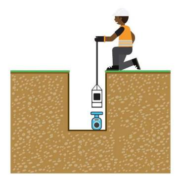
NC2 Vertical direct unobstructed access with continuous attachment to a person riding hoist or similar mechanical rescue device.
