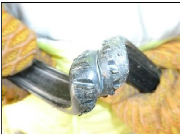
Figure 1: Identifying defects in external beads, brittle split evident on twisting
