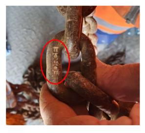
Please check all your lifting chains and if you discover a set of 'FORCE' brand chains they are to be quarantined immediately. 'FORCE' chains can be identified by the logo stamped onto a link or several links along the chain.
